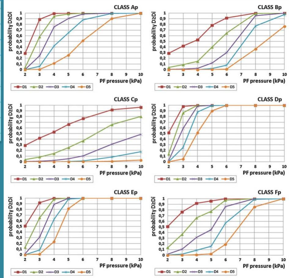
For each structural class Ap-Fp, vulnerability functions have been defined (Zuccaro et al., 2008). As for the ash fall case, they have been determined through a **hybrid method based** on typological analysis of about **90,000** buildings surveyed in the Vesuvian area (Spence et al. 2004a, b; Zuccaro et al. 2008)
