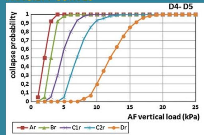
For each vulnerability class in the Vesuvian area, ash fall fragility curves have been calculated through a **hybrid method** characterized by the following steps:
