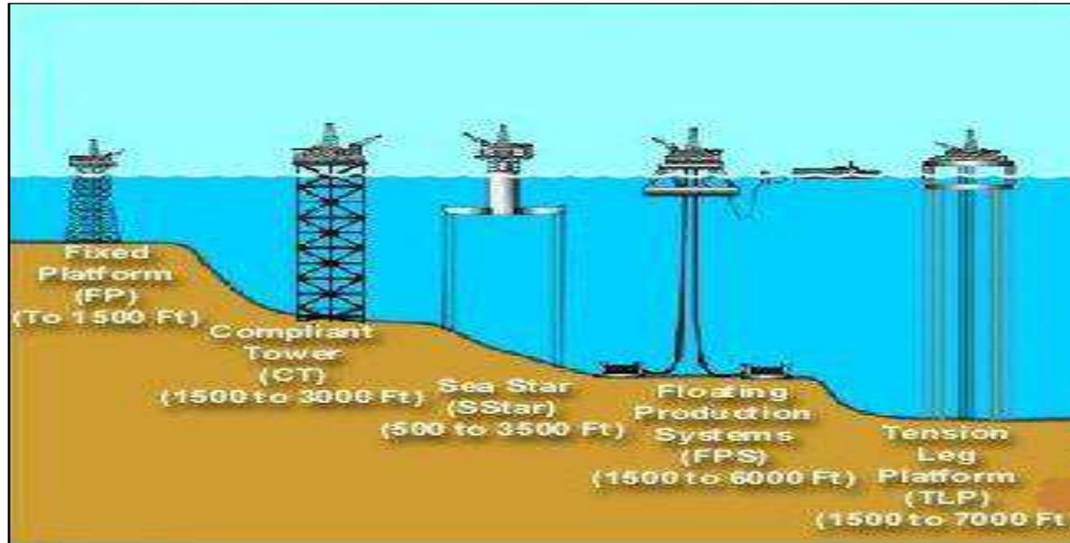
Offshore projects are denoted by offshore facilities for drilling and extracting hydrocarbons. Fixed or floating platforms can be used, depending on water depth. The extracted hydrocarbons are then transported onshore through a sea line-system
