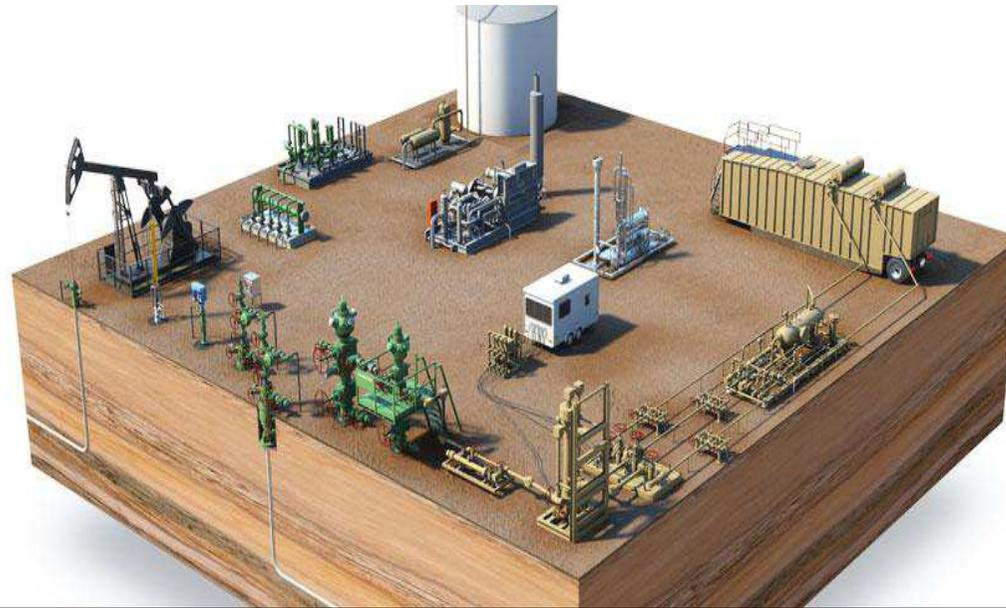
Onshore projects are characterized by the construction and installation of on-shore facilities. The liquid and/or gas hydrocarbons extracted from the wells are firstly stored and then the liquids are sent through flow-lines to a preliminary treatment unit and then to a refinery. The gas follows a similar process until the preliminary treatment; afterwards it is sent for further treatment through a gas pipeline
