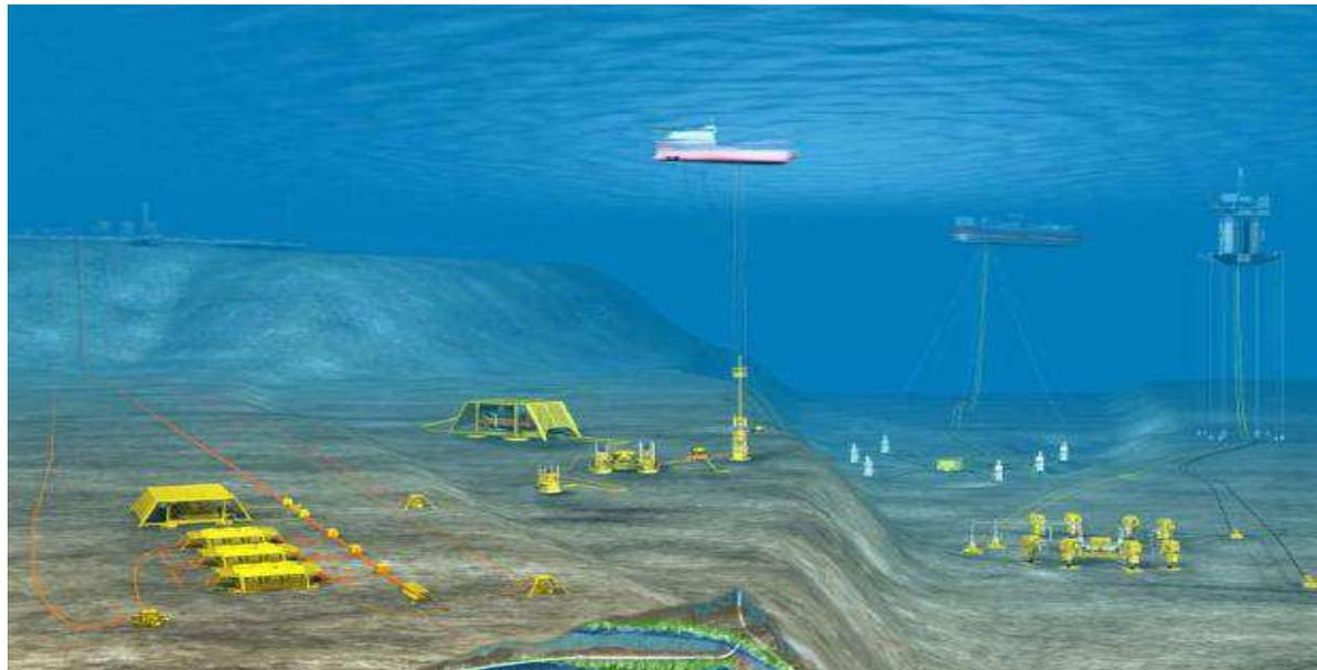
Subsea projects are characterized by undersea facilities for extraction and production. The need to install undersea facilities is due to the technical or economical infeasibility of utilizing offshore platforms. When there are more than one undersea wells, the wells are interconnected through flow lines, in addition to the sea-lines that link the wells of extraction and production with onshore facilities
